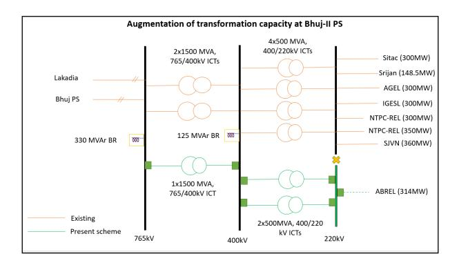
Fig-1: Augmentation of transformation capacity at Bhuj-II PS
